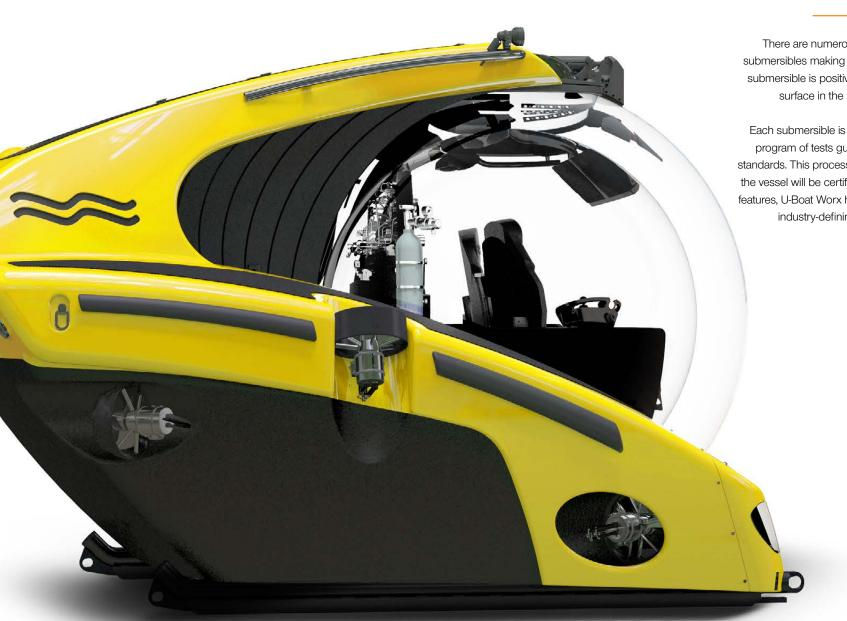
There are numerous tiers of safety built into all U-Boat Worx submersibles making them the safest in the world. For example, the submersible is positively buoyant and will float automatically to the surface in the highly unlikely event of a power failure.
